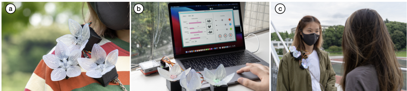
Figure 1: The Emolleia Prototype. (a) shows the kinetic flower display worn by a user (the system is self-contained), (b) the interface over which the user can define the animated motions and colors, (c) depicts Emolleia in a social interaction context.
