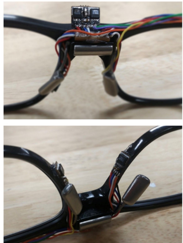
Figure 1: Experimental prototype with two pairs of sensors for the forehead area (top) and nose (bottom).
