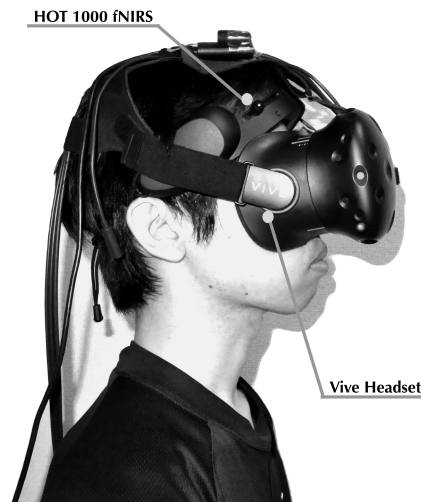
Figure 1. Experimental Setup: Participant wearing the VIVE VR headset and an fNIRS (the HOT-1000 from Hitachi connected to the computer over Bluetooth).
