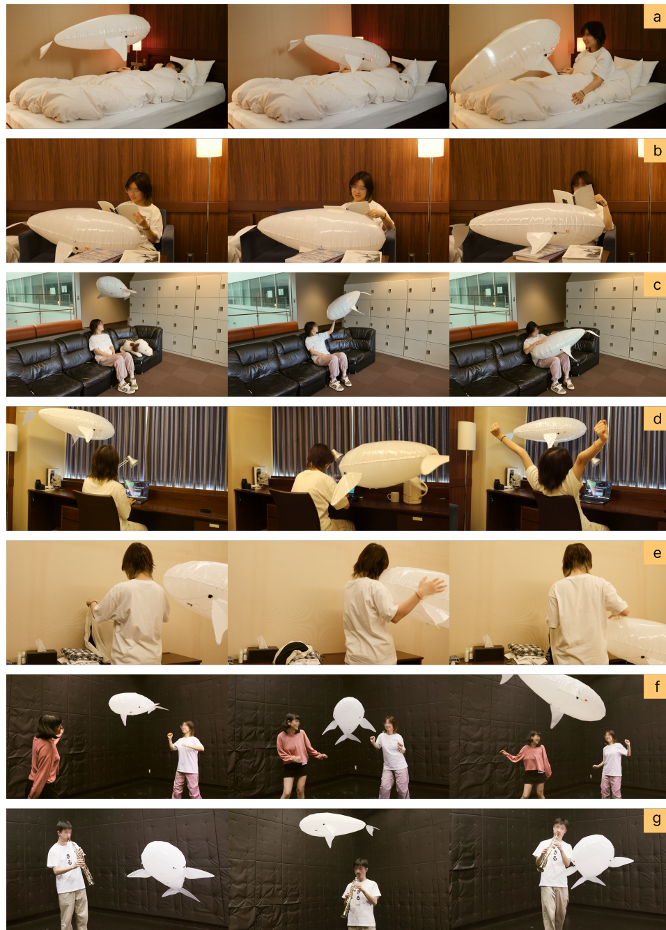
Figure 16: Proof-of-concept demonstrations illustrating how the proposed design principles guide interaction design: (a) Gentle wake-up: The SFR hovers above a user and contacts at a set time, offering a calm alternative to traditional alarms. (b) Dynamic reading support: While the user reads on a sofa, the SFR rests on the lap as an inflatable book stand, adjusting naturally to posture. (c) Tactile comfort: The robot approaches a waiting user, who holds and interacts with it, alleviating boredom and loneliness. (d) Well-being intervention: To counter sedentary behavior, the robot approaches a desk-bound user, delivering a gentle shoulder nudge and hovering to invite movement. (e) Companionship in mundane tasks: as a user folds laundry, the robot floats nearby, transforming a routine chore into an engaging experience. (f) Expressive dance partner: During music and dance, the robot synchronizes wing flaps with the rhythm, encouraging social play and easing awkwardness. (g) Music companion: While the user plays an instrument, the remote operator adjusts the robot's flight path and wing motion to match the musical tempo.
