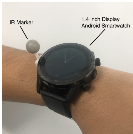
Figure 4: Smart watch prototype equipped with IR Marker
