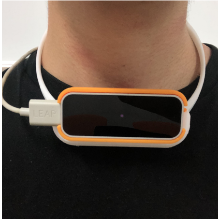
Figure 5: Tracking camera attached to the neck
