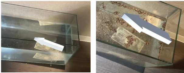
Figure 4: Testing Image targets (1000 yen bill) in no-turbidity (left) and high turbidity (right) environments
