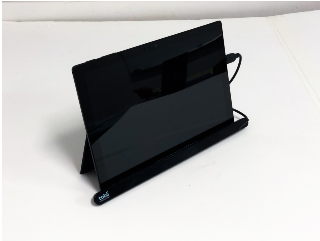
Figure 2: The demonstration system. A Windows tablet with Tobii 4C attached.
