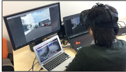
Figure 1: (a) Installed eye trackers on the HTC Vive, (b) GazeSphere system using head rotation for navigation, and (c) scene during navigation with virtual cue and semi-transparent rendered video
