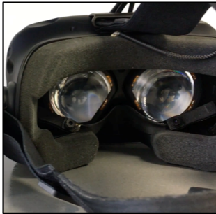
Figure 1: (a) Installed eye trackers on the HTC Vive, (b) GazeSphere system using head rotation for navigation, and (c) scene during navigation with virtual cue and semi-transparent rendered video
