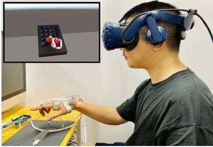
Figure 6: The study setup : Evaluating SMA springs with Input test In Virtual Reality Environment
