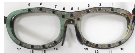
Fig. 8. The placement of photo-reflective sensors
