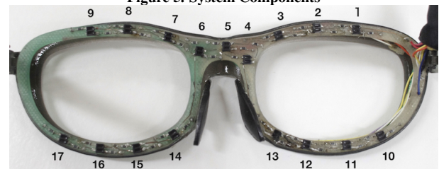
Figure 6. The Placement of Photo Reflective Sensors
