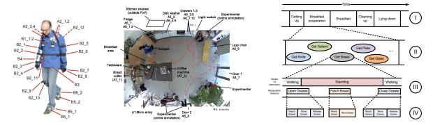
Figure 1: Experimental Setup for the "Everyday living" dataset. On the left, the on-body sensing setup is shown. The picture in the middle depicts the sensors in the environment. On the right, you see a part of the hierarchical activities performed by the test subjects. The experiments were recorded for the Opportunity EU Project. (Roggen, Calatroni, and Rossi 2010)
