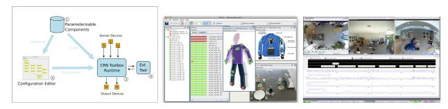
Figure 2: The Context Recognition Network toolbox concept on the left shows a repository of combinable components. The monitoring tool in the middle helps to keep track of sensor failures etc. during recordings. The labeling tool on the right helps to assign context labels and readjust sensor data in post-processing. All software is made available as open source (Bannach and Lukowicz 2011).
