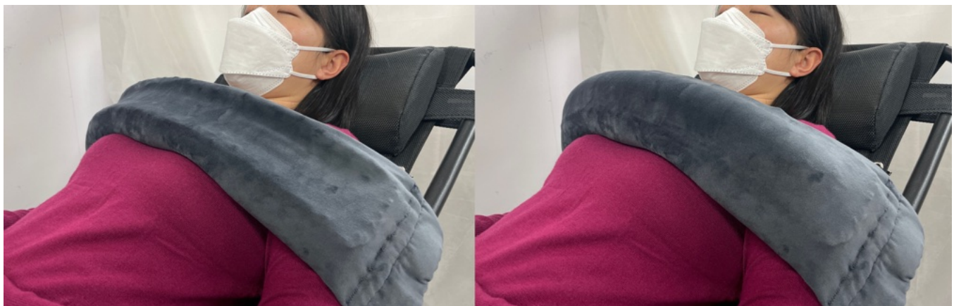
Figure 1: Movement of MindSpace captured still - Exerting tactile sensation of life-like breathing movement with squeeze-like deep touch pressure on users' upper chest area.
