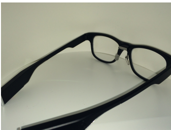
Figure 2: The glasses prototype: There are the 3 electrodes around the nose used for eye movement analysis (EOG).
