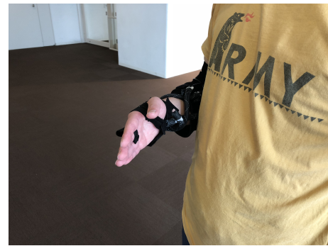
Figure 1: The Artificial Muscle sleeve is a soft exoskeleton that enables the user to obtain information or skill through their body. In assisting navigation scenarios, users can feel a slight drag towards the direction he/she is suppose to take.
