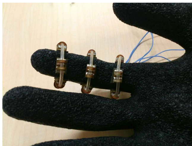
Figure 1. The prototype of a whole-finger haptic device with 3 SMA wire rings
