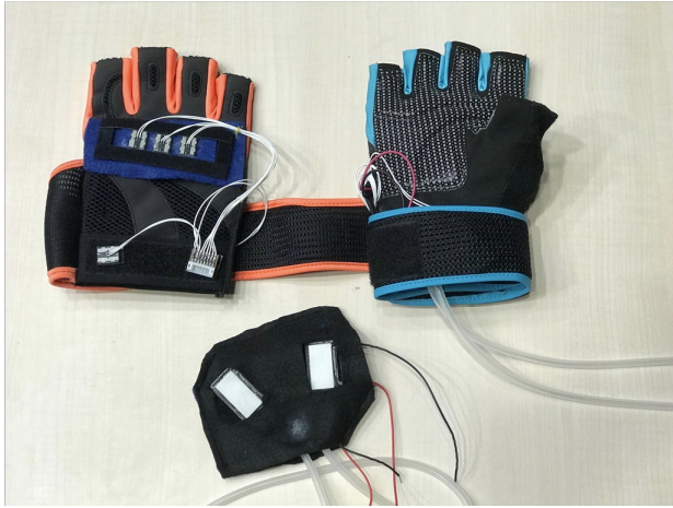
Figure 2: Prototype of the thermal feedback glove with 2 Peltier elements and water cooling.
