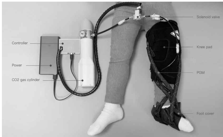
Figure 1: Our PGM system being used to help a boy with cerebral palsy stretch his left plantar flexor muscle.
