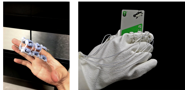
Figure 1: We investigated different parameters to emulate a haptic feedback on user's hand (depicted right). Our target audience at this stage is researchers and experimenters interested in cognition and perception. In this setup, our objective was to evaluate how can the participants perform cognitive tasks, such as getting informations from daily life objects. The early prototype is depicted on the left.
