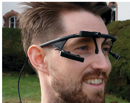
Figure 2. PUPIL from Pupil Labs is an accessible, affordable, and extensible open source platform for head-mounted eye tracking, mobile gaze-based interaction, and egocentric vision research.
