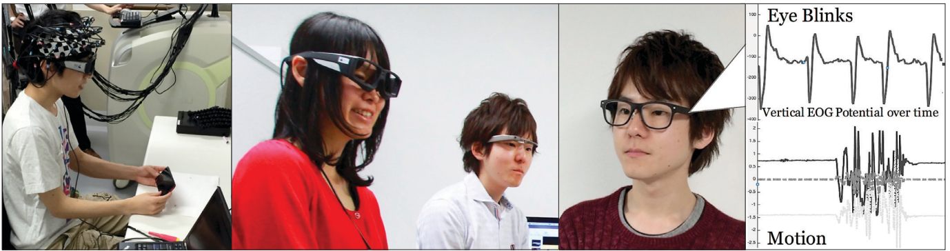
Figure 1. From fNIRS and mobile eye tracking glasses to Google Glass to unobtrusive smart glasses (J!NS MEME prototype recording eye and head movements).
