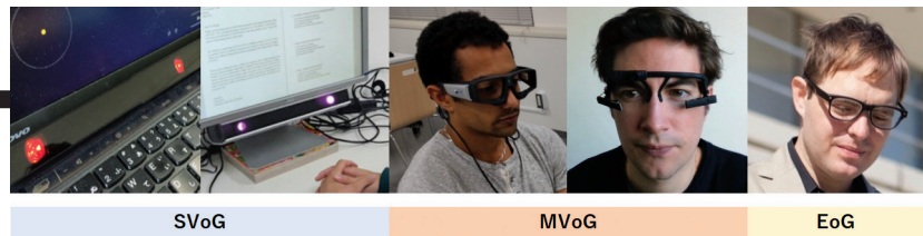
FIGURE 1. Different kinds of eye trackers (left to right): two stationary video-oculography systems, two mobile video-oculography systems and one electro-oculography system.
