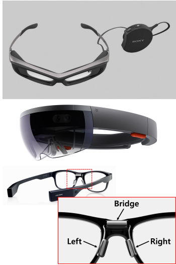
Figure 1: Examples of commercial Smart Eyewear. Sony Smart glasses, Microsoft HoloLens, JINS MEME.
