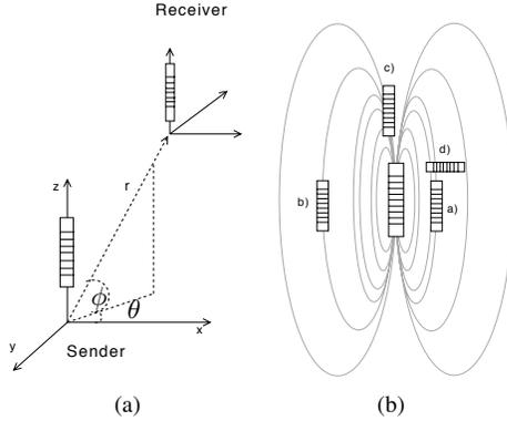
**Figure 1.** (a) Orientation and Distance overview. (b) Schematic Magnetic field with receiver coils.
