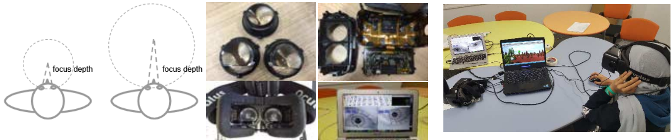
Figure 1. (a) Focus depth of the user where left is close and right is far, (b) Custom hardware, integrating a pupil labs tracker into Oculus, and (c) Experimental setup
