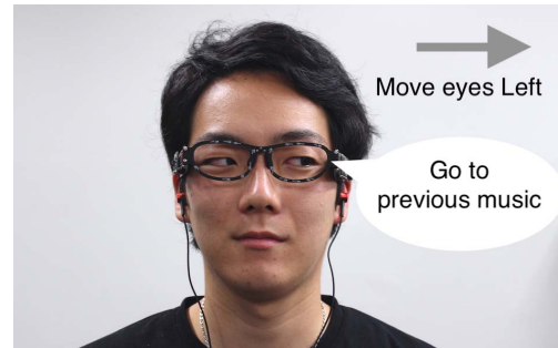
Figure 1: We defined face-related gestures used to perform daily tasks in an elicitation study. Then, we verified the gestures’ technical feasibility using smart eyewear.
