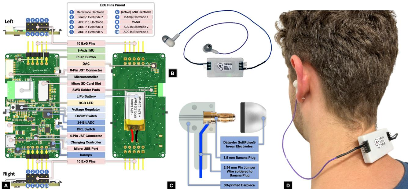
**Figure 2:** (A) PCB and components of OpenEarable ExG; (B) 3D-printed in-ear plugs based on Dätwyler SoftPulse in-ear electrodes [10] (C) assembled device with 3D-printed housing and custom in-ear electrodes; (D) user wearing OpenEarable ExG.
