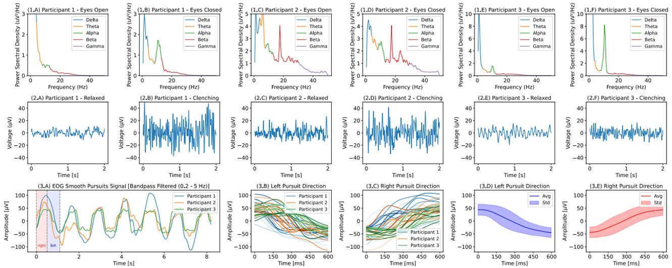
**Figure 3: (1.A) - (1.F) display brain activity measured via ear EEG for three participants, with eyes open and closed, revealing increased alpha activity when eyes are closed. (2.A) - (2.F) illustrate the rise in signal amplitude measured by ear EMG during jaw muscle clenching for the same participants. (3.A) - (3.E) present smooth pursuit signals measured via ear EOG, showing signal deflection in opposite directions based on the participants' gaze direction.**
