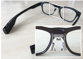
Figure 3: The settings of electrodes to calculate EOG vertical and horizontal component on J!NS MEME.
