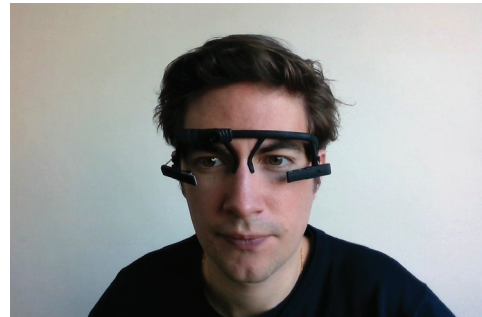
(b) Pupil mobile eye tracker, an open source and inexpensive device.
