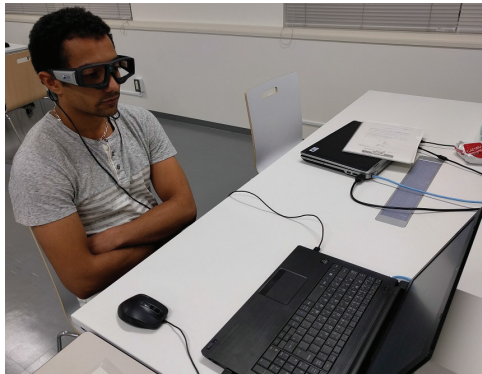
(a) SMI mobile eye tracker, a professional eye tracker.
