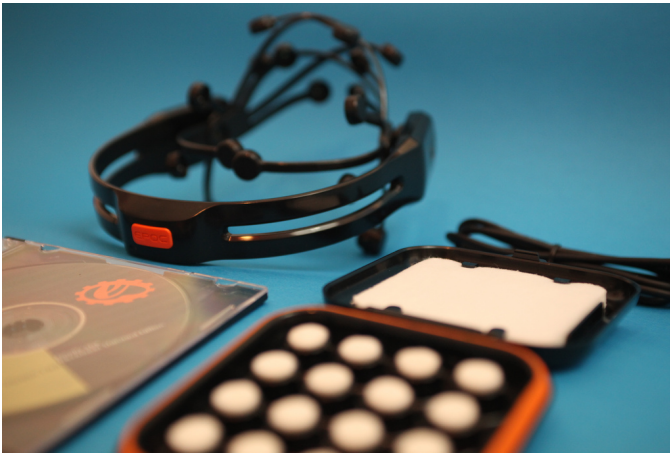
Fig. 2. The Emotiv EGG system used for the experiments.
